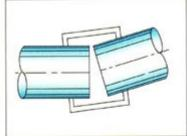
YN-Multiflex pipe couplings allow a maximum inclined deviation of 10°
