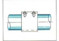
The coupling acts as a flexible compensator for movements caused by heat and also effectively dampens vibration.
