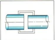
The difference in diameters between the pipes to be joined maybe 4mm and the coupling is subitable for all piping materials,
