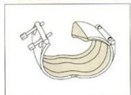
Suitable for new building and repair work, The piping can be quickly disassembled and the couplings can be used again.
