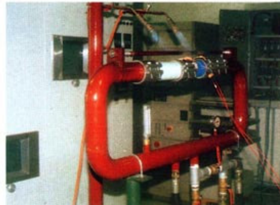
TEST CONTENT:PERFORMED 30MIN BY G.L RULE AT 800°C 5.0kg/cm 2 CIRCULATION
